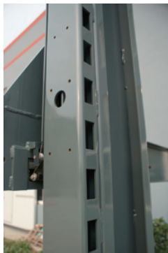
- Dynamic locking device With 6 locking tabs
